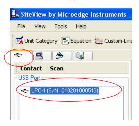
Double click on the icon to start the communication with the data logger. On the success of the communications, the status page of the logger will be displayed on the right side area.
